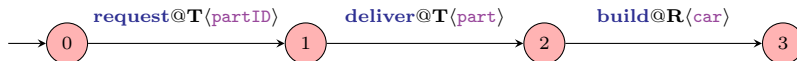
Figure 3: A Factory protocol that can interface with the Warehouse using the Transport role.
